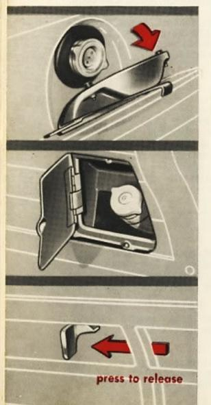
WARNING: Don't allow flames or sparks to be brought near the battery vent openings or the fuel tank filler. Explosive gases are produced during normal battery operation, and dangerous gasoline vapors may be present at the fuel tank filler when the cap is off and gasoline is being pumped into the tank.
