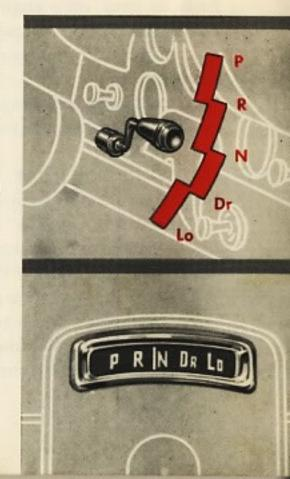
DRIVING ON SAND, SNOW, OR ICE. When you're driving through deep sand or snow, shift into second or low gear (Lo on Fordomatic). You'll have more power available to keep you going steadily at low speed without overworking the engine.
