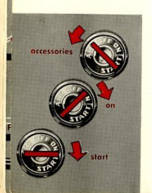
IGNITION SWITCH. When the key in the ignition switch is in the OFF position, the ignition, gauges, indicators, and electrical accessories (radio, heater, etc.) won't operate. Turn the key to ACC at the left, and you can operate the accessories when the engine is stopped. When you turn the key to ON, the ignition and gauges as well as the accessories can be used. Turning the key, against a spring tension, toward START at the extreme right operates the starter.
