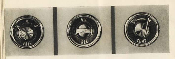
FUEL GAUGE. You can tell how much gasoline is in the fuel tank by looking at the fuel gauge. The gauge pointer rests at the E (empty) mark when the ignition is off.
