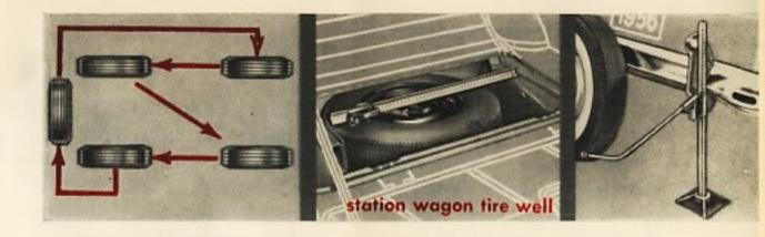
TIRES. Check your tires, including the spare tire, frequently to be sure that the tire pressures are correct. To equalize tire wear, cross-switch all five tires every 5000 miles, following the pattern shown in the illustration on this page. Each time your tires are cross-switched, you should have all the wheels of your car checked for proper balance.
