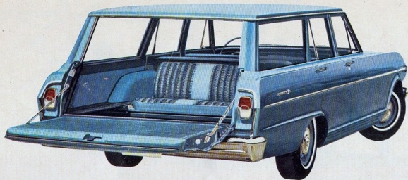
CHEVY II 300 4-DOOR 3-SEAT STATION WAGON SHOWN IN TWILIGHT TURQUOISE. Third seat faces rear, easy to enter, no crawling over a second seat. Power-operated rear window is standard equipment. (Optional at extra cost on Nova 400 and Chevy II 100.)
